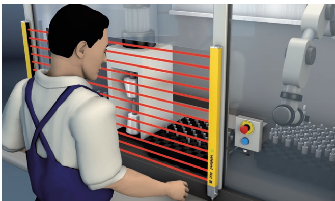
Finger, hand and arm protection on machines with the safety light curtain SLC
